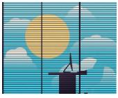
Sunny weather, occupant not present: Artificial lights are off, blinds are covering direct sunlight to minimize cooling needs.
